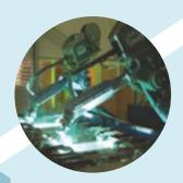
Step 07: Friction Stir Welding
